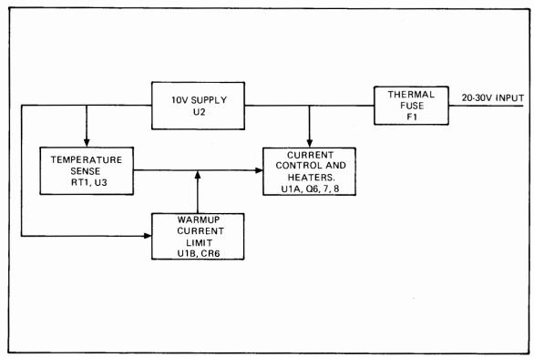
Figure 8-14. Oven Controller Block Diagram
