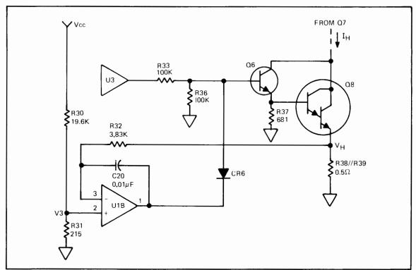
Figure 8-11. Turn-on Current Limit Circuit
