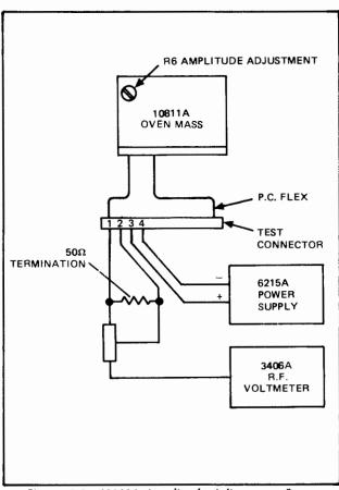
Figure 5-2. 10811A Amplitude Adjustment Set-up
