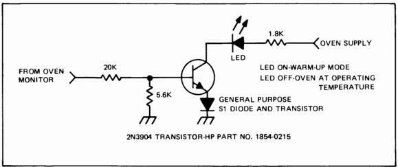
Figure 2-2. Oven Monitor LED Circuit
