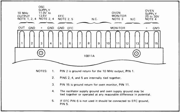
Figure 2-3. 10811A Supply and Output Connections
