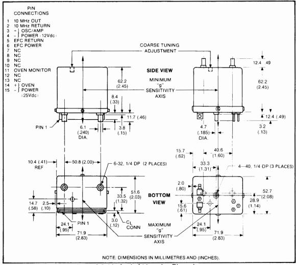
Figure 2-5. Mechanical Mounting Dimensions
