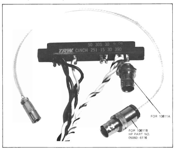
Figure 8-13. 10811A/B Special Test Connector
