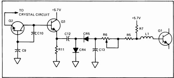
Figure 8-7. Automatic Gain Control (AGC)
