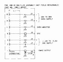
Figure 8-15. 10811A/B Oscillator Schematic Diagram
