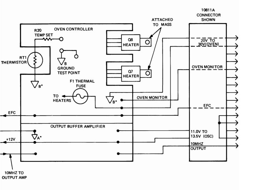
Figure 8-2. 10811A/B Overall Block Diagram
