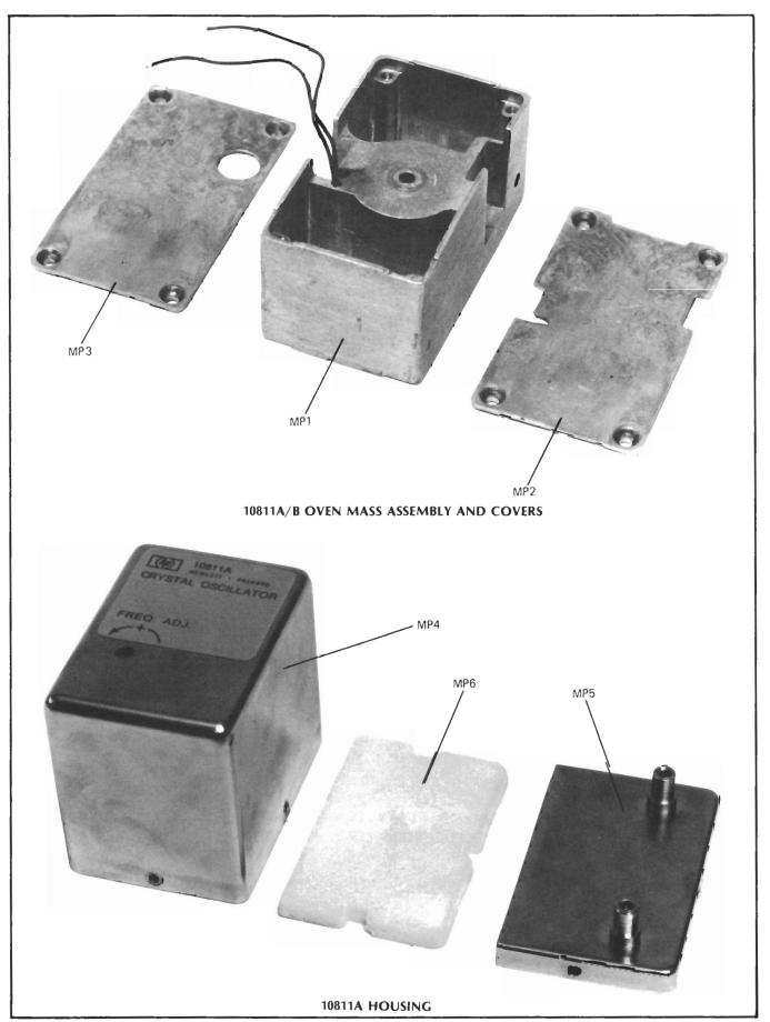
figure 6-1. Mechanical Parts
