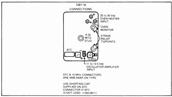
Figure 2-4. 10811B Supply and Output Connections
