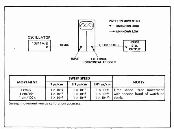
Figure 5-1. Oscillator Adjustment Setup
