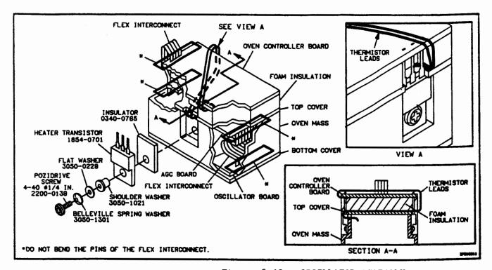
Figure 8-13a. OSCILLATOR ASSEMBLY
