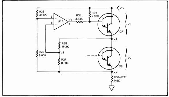
Figure 8-12. Heater Transistor Balance Circuit
