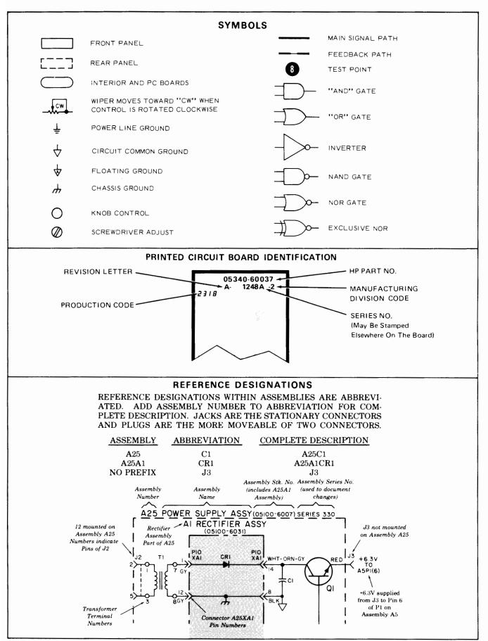
Figure 8-1. Schematic Diagram Notes
