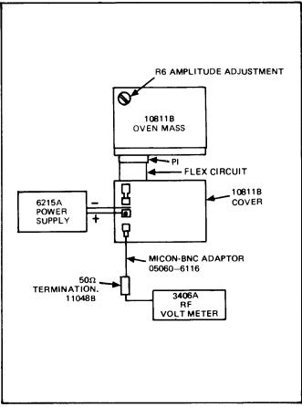
Figure 5-3. 10811B Amplitude Adjustment Set-up
