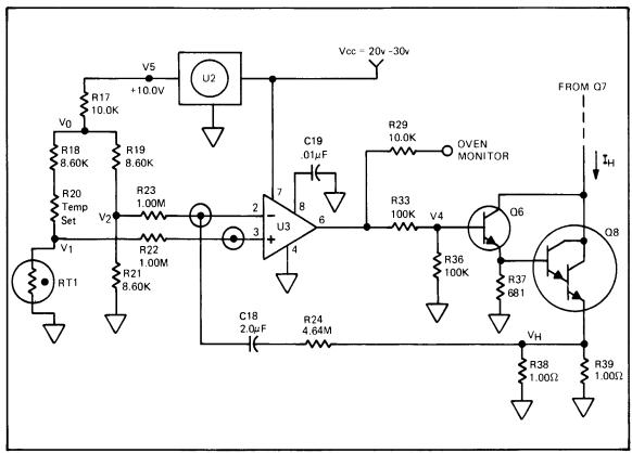
Figure 8-10. Oven Control Circuits
