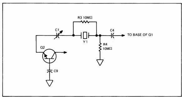
Figure 8-5. Frequency Tuning Circuit
